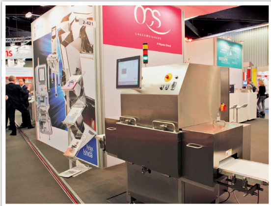
Combined X-ray scanner/ check- weigher SCW 3000-C-C- CF by OCS Check- weighers
