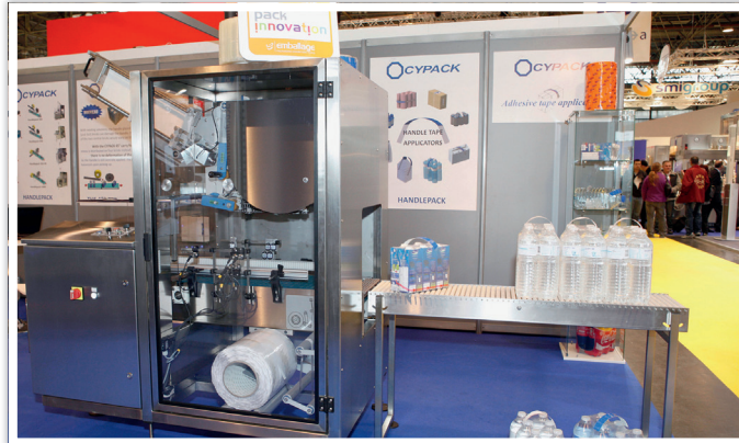
Patented Handlepack 450 by Cypack even realizes the application of carry handles in 45° angle
