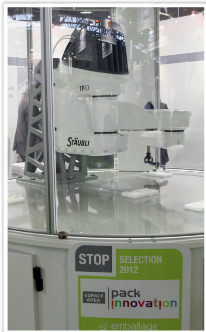
TP80 fast Picker robot by Stäubli
