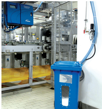
The pelletized adhesive is automatically supplied from an external 60 kg container
