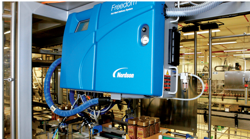
The central component of the Freedom system is the melter. Photos: Kimberly Wittlieb
