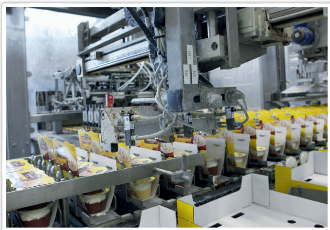
Three MiniBlue II hotmelt applicators built up in a row
