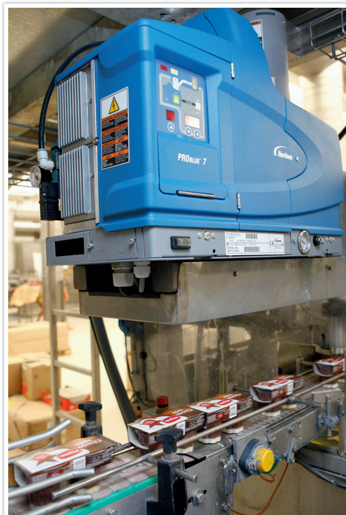
Automatic, sensor-controlled hotmelt filling system of ProBlue Fulfill series
