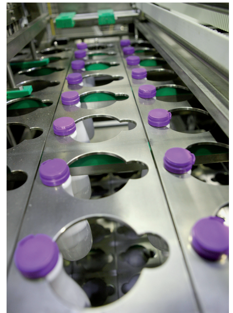
Special cell boards allow to handle two different neck diameters (photo: Kimberly Wittlieb)
