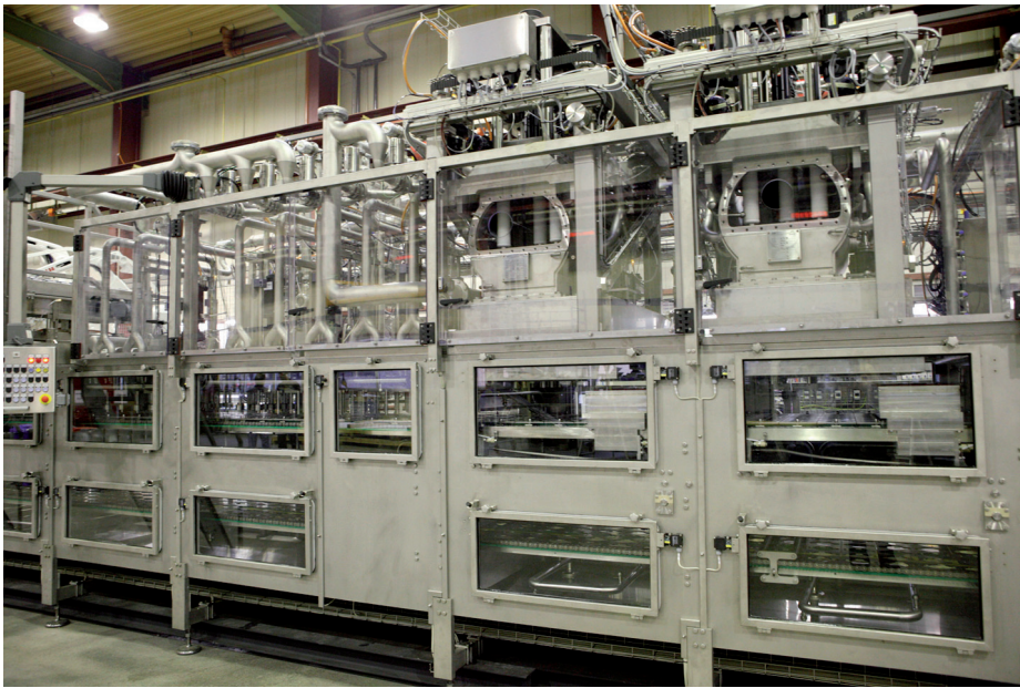
The bottle sterilization section (left) is followed by a pair of dosing systems (photo: Kimberly Wittlieb)
