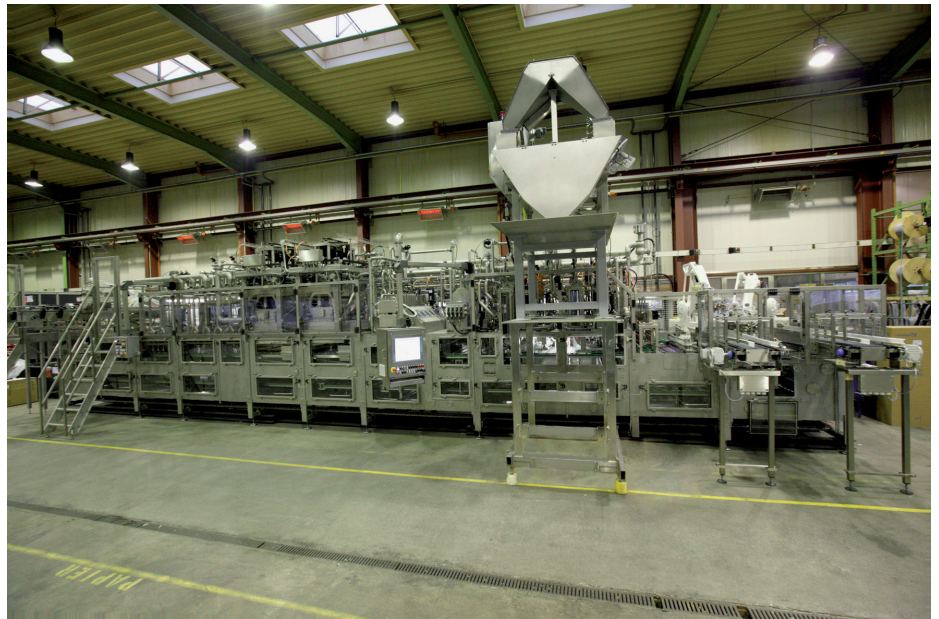
Overall view of the 5200-8/8 FF plastic bottle filling and sealing machine designed for Unilever in the Ahaus plant shortly before shipping (photo: Kimberly Wittlieb)
