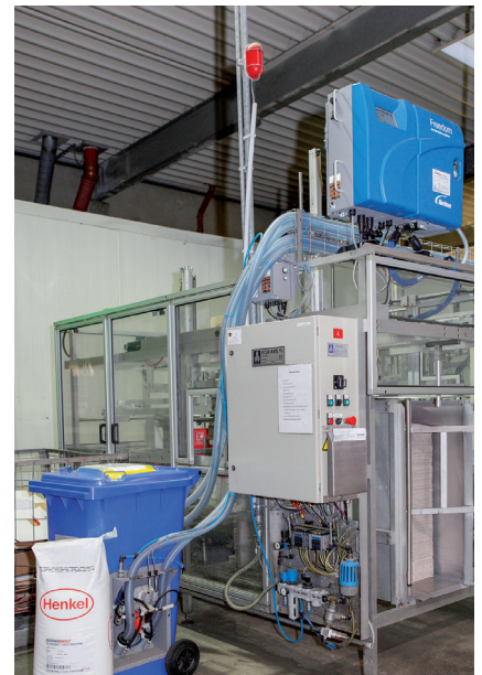
The 240-liter storage tank is equipped with a multiple-feed system for supplying granulate to as many as four adhesive melters
