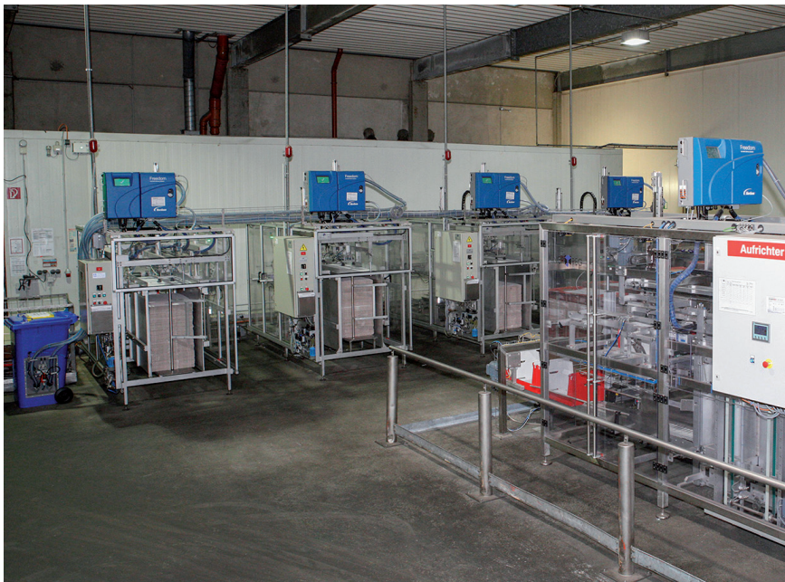
Bottom trays are produced and distributed to the production lines with five box erectors simultaneously in potato chip production
