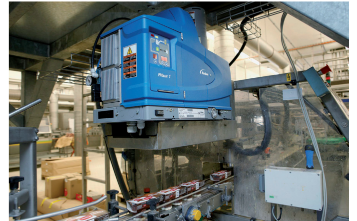
Automatic, sensor-controlled hotmelt filling system of ProBlue Fulfill series.
