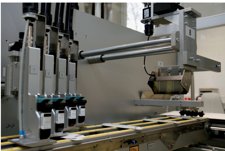
The core of the system is the printing section with four movable or cascading print heads and printing inspection via camera.
