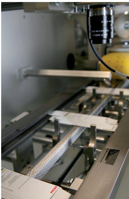
Before the printing process, the pharma code is verified by means of camera inspection.
