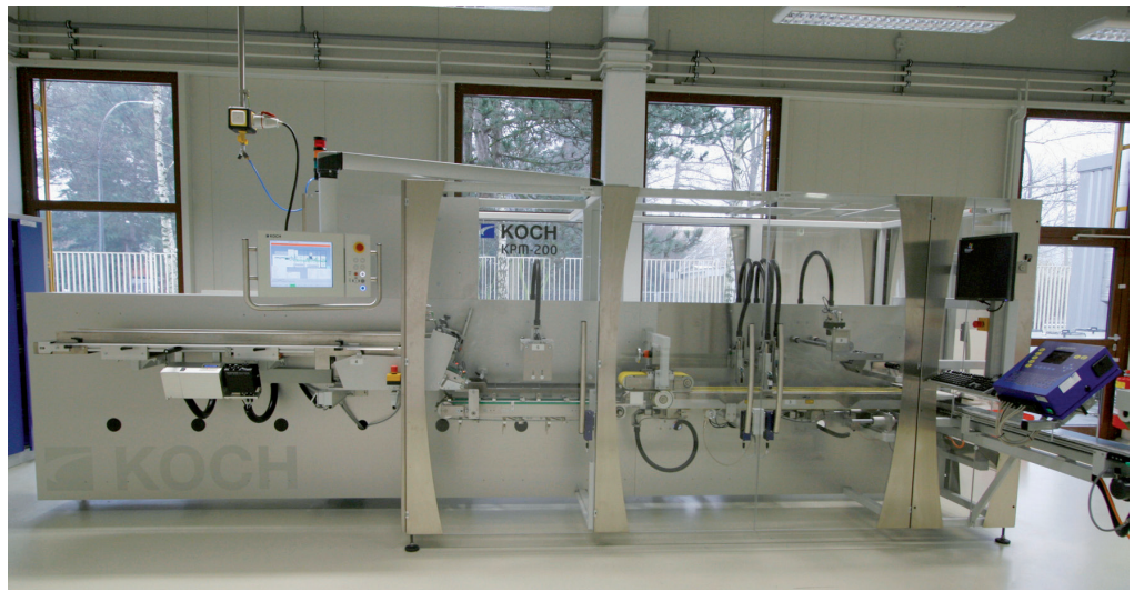
The KPM-200 offline identification machine including the product erecting and grouping systems.
