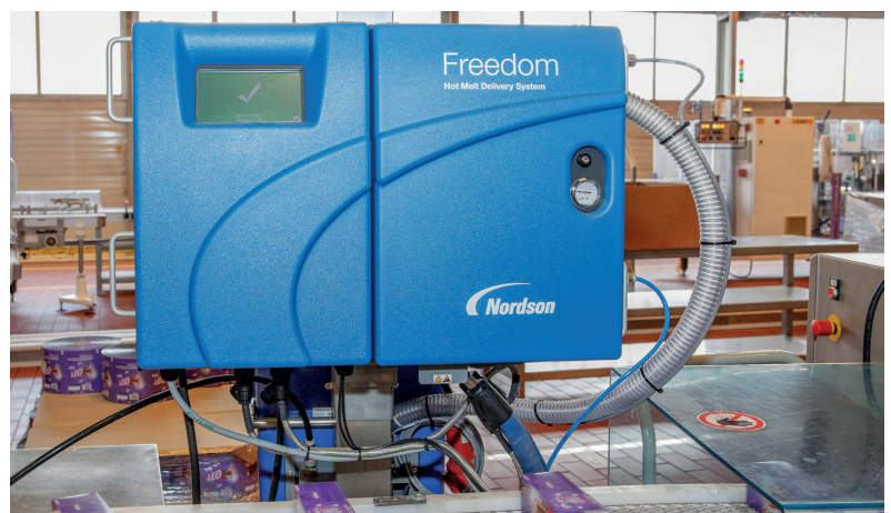
The Freedom tankless hotmelt application system has been installed at head height above the product outfeed belt.
