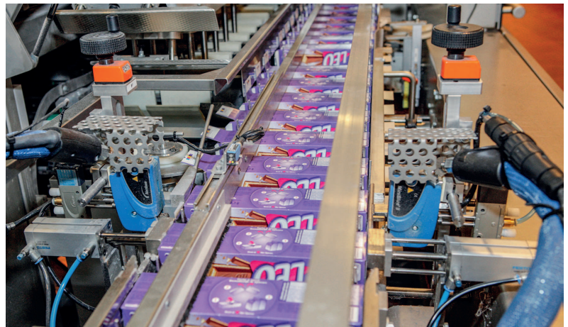
Two self-cleaning applicators of the new MiniBlue II SureBead type apply two adhesive dots to each side.
