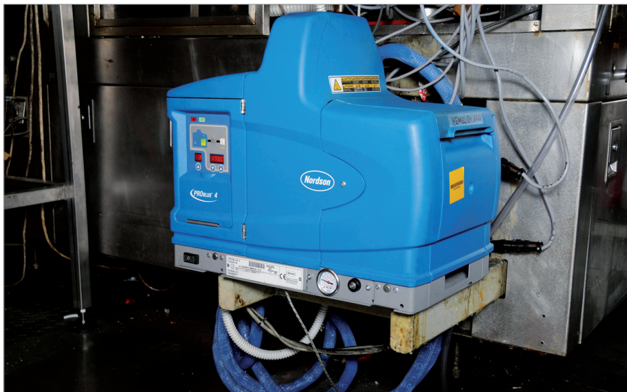
A ProBlue 4 melter unit is used to heat the hot-melt.
