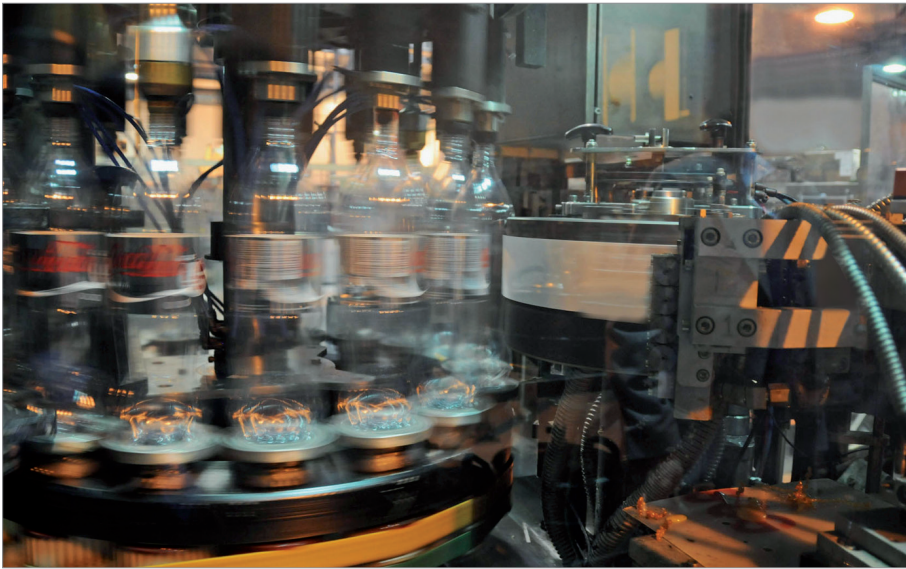
The labeling stations typically run in production with a speed of 24,000 and 20,000 bottles per hour respectively.
